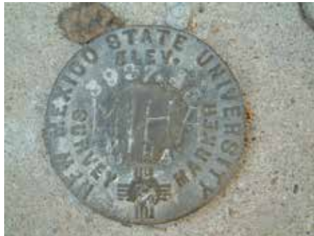
Elevation marker found next to the steps of the northeastern entrance to the building.
